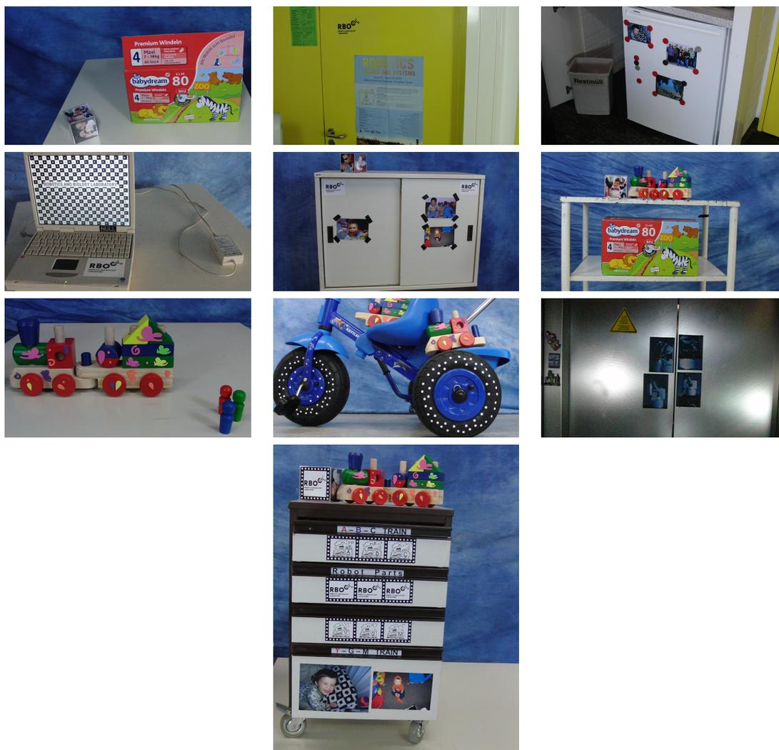
**Figure 10.2.** Ten real-world objects. Our robot has interacted with and modeled these objects. The objects differ in size, shape, color, texture and their kinematic structure. Modeling their shape and kinematic structure provides the robot with necessary information for manipulation.
