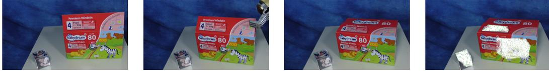
**Figure 10.3.** Identifying rigid bodies: box. Left to Right: The first column shows the box before the interaction; the second column shows the interaction itself; the third column shows the box after the interaction; and the fourth column shows the results of segmenting the graph of tracked features into clusters of features, where each cluster is associated with a different rigid body. Note how small the overall motion of the box is.
