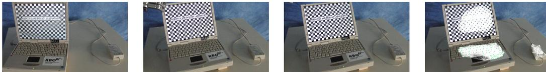
**Figure 10.9.** Identifying rigid bodies: laptop. Left to Right: The first column shows the laptop before the interaction; the second column shows the interaction itself; the third column shows the laptop after the interaction; and the fourth column shows the results of segmenting the graph of tracked features into clusters of features, where each cluster is associated with a different rigid body.
