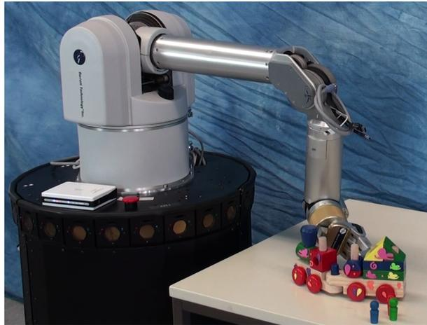
**Figure 10.1.** Interacting with a toy train. Our Mobile Manipulator interacts with a toy train, and identifies a set of rigid bodies: train engine, train car, and wooden figures. These rigid bodies are segmented from the background throughout the interaction.
