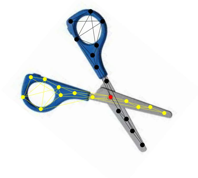
**Figure 6.5.** The highly connected subgraphs and rigid bodies analogy. The scissors is composed of two rigid parts. Identifying the highly connected sub-graphs (yellow and black) is analogous to identifying the object’s different rigid bodies. The intersection between the two clusters indicates the location of the revolute joint (red dot).
