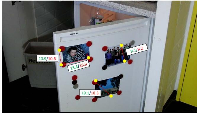
**Figure 8.1.** Quality of three-dimensional reconstruction. Yellow circles mark a few selected features on the fridge. Four 3-D distances are labeled by red dashed lines. Distances are showed in green (manual measurements) and red (computed by the reconstruction algorithm). They are consistent.
