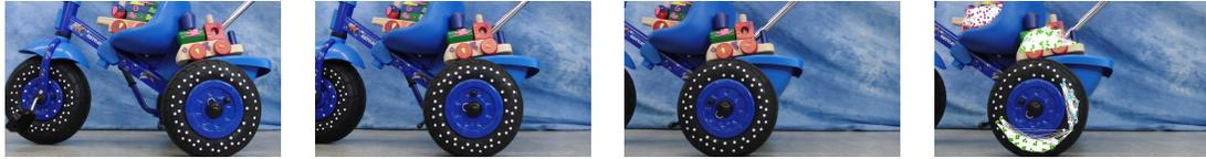
**Figure 10.17.** Identifying rigid bodies: tricycle. Left to Right: The first column shows the tricycle before the interaction; the second column shows the interaction itself; the third column shows the tricycle after the interaction; and the fourth column shows the results of segmenting the graph of tracked features into clusters of features, where each cluster is associated with a different rigid body.
