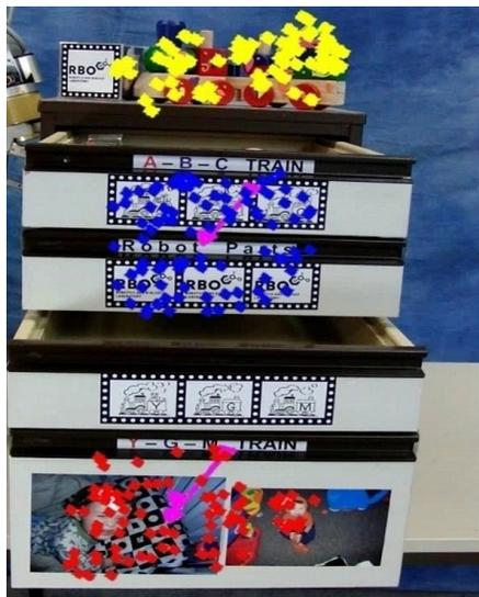
**Figure 10.22.** Detecting the kinematic structure of a set of drawers. Three clusters are detected; the cabinet’s top (yellow), the top drawer (blue), and the bottom drawer (red). The three detected prismatic joints are marked in pink.
