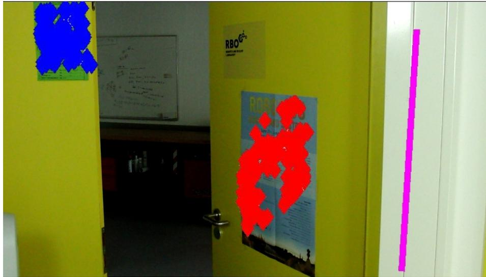
**Figure 10.6.** Detecting the kinematic structure of a door. Two clusters are found; a static cluster on the frame of the door (blue), and the door itself (red). A revolute joint (pink) between the door and its frame is found.
