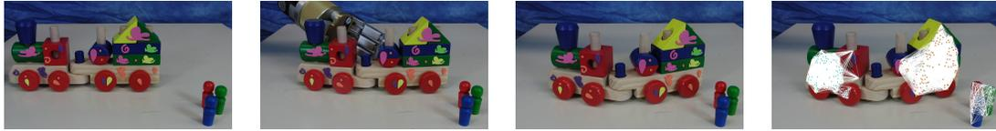
**Figure 10.15.** Identifying rigid bodies: toy train. Left to Right: The first column shows the train before the interaction; the second column shows the interaction itself; the third column shows the train after the interaction; and the fourth column shows the results of segmenting the graph of tracked features into clusters of features, where each cluster is associated with a different rigid body.
