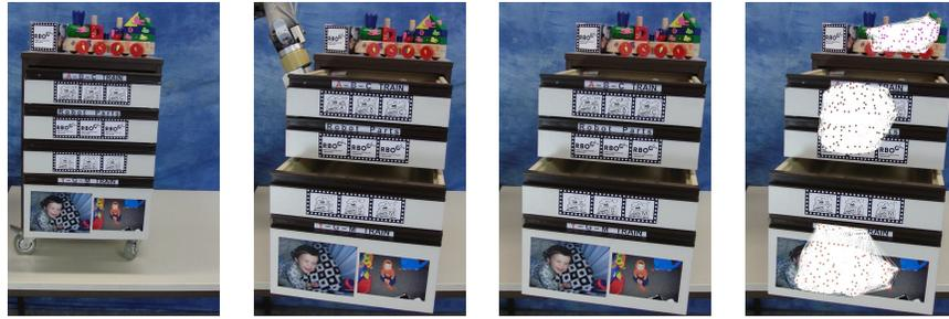
**Figure 10.21.** Identifying rigid bodies: set of drawers. Left to Right: The first column shows the drawers before the interaction; the second column shows the interaction itself; the third column shows the drawers after the interaction; and the fourth column shows the results of segmenting the graph of tracked features into clusters of features, where each cluster is associated with a different rigid body.
