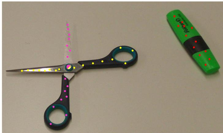
(c) Relative motion observed between the scissors's parts. Features are finally clustered into three rigid bodies (red, yellow and pink dots). The revolute joint is indicated by a larger dot.
