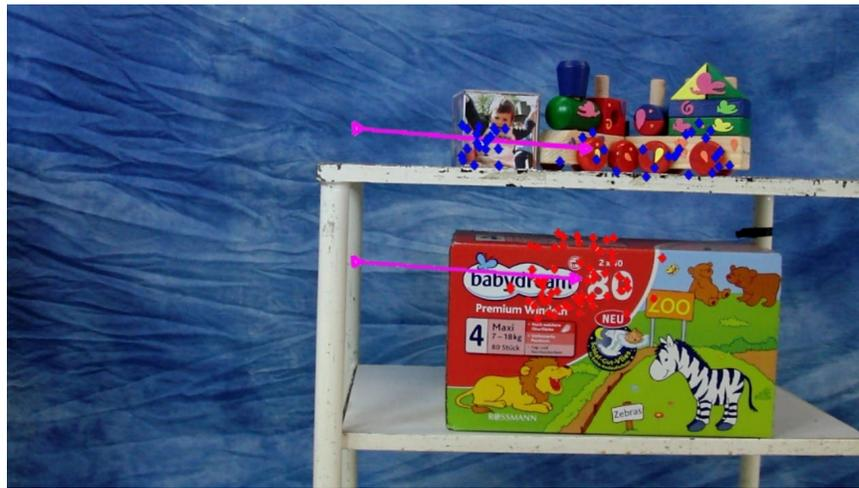
**Figure 10.14.** Detecting the kinematic structure of a shelf on wheels. Two clusters are detected; the top shelf (blue), and the bottom shelf (red). Two prismatic joints (pink) are found: one joint is between the top shelf and the background, and the second is between the bottom shelf and the background. The skill correctly determines the two shelf clusters to be rigidly connected, but has low confidence because the train moved slightly.
