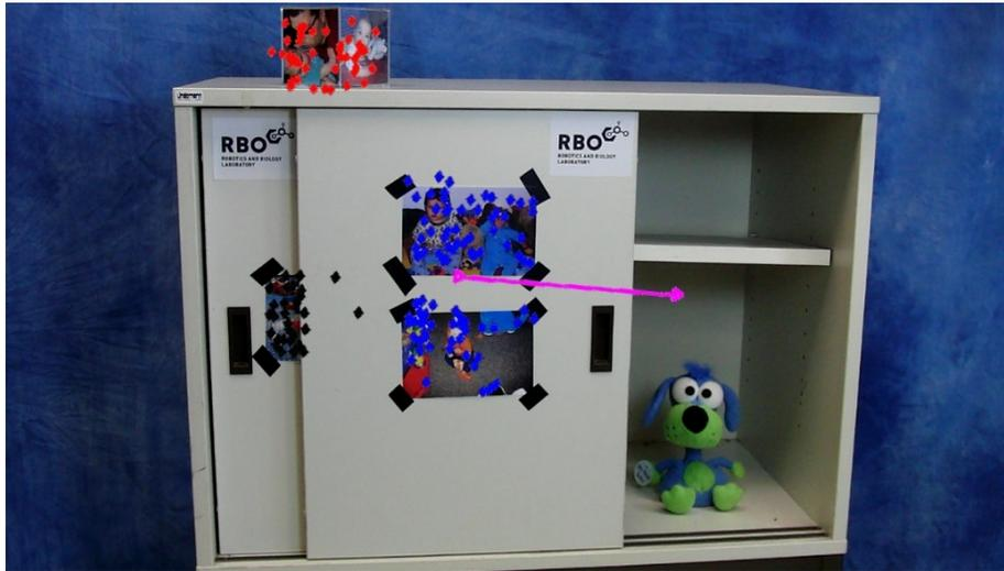
**Figure 10.12.** Detecting the kinematic structure of a cupboard. Three clusters are detected; the right door (blue), the left door (black) and a static background cluster associated with the picture cube (red). A prismatic joint (pink) between the right (moving) door and both the left (static) door and the picture cube is found. Both axes are shown in the figure (overlapping). A rigid connection is detected between the two static clusters (left door and picture cube).
