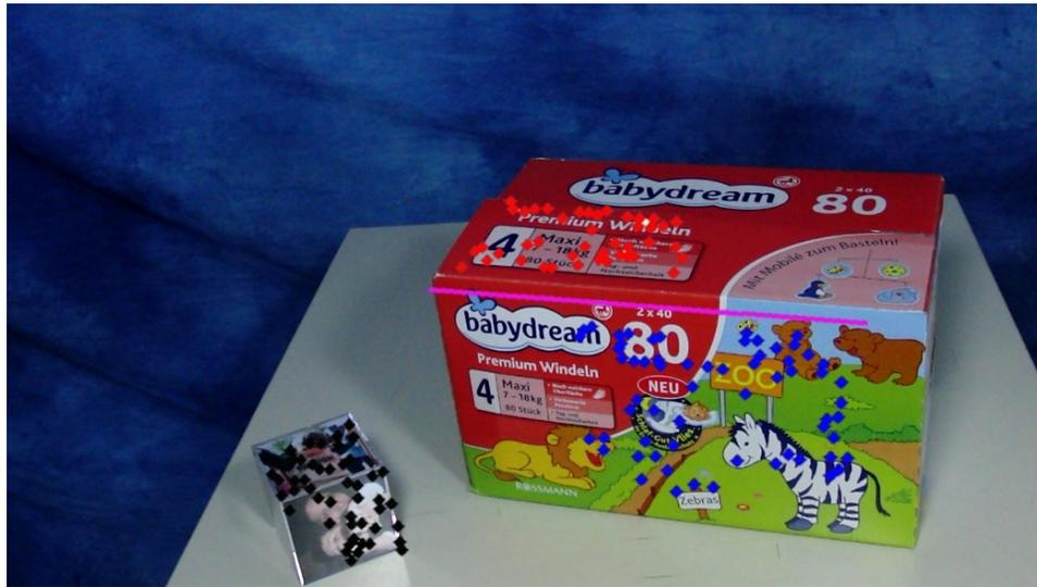
**Figure 10.4.** Detecting the kinematic structure of a box. Three clusters are found; a static cluster on the picture cube (black), the body of the box (blue), and the top flap (red). A revolute joint (pink) between the body of the box and the top flap is found.
