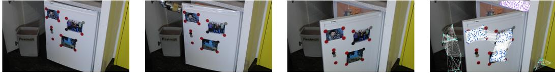
**Figure 10.7.** Identifying rigid bodies: refrigerator. Left to Right: The first column shows the refrigerator before the interaction; the second column shows the interaction itself; the third column shows the refrigerator after the interaction; and the fourth column shows the results of segmenting the graph of tracked features into clusters of features, where each cluster is associated with a different rigid body.
