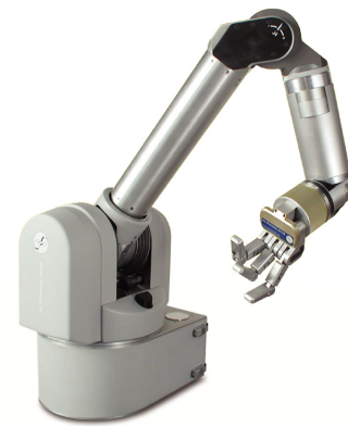
Fig. 5. Barrett Technologies Whole Arm Manipulator (WAM)
