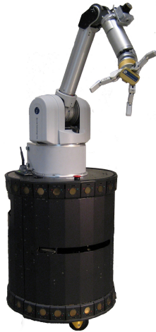
Fig. 5. UMan (UMass Mobile Manipulator)
