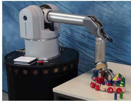
Fig. 1 Our Mobile Manipulator interacts with a toy train. To extract a kinematic model of the train, it first segments a set of rigid bodies from the background: train engine, train car, and wooden figures. This segmentation is then used to estimate the 3D shape and motion of the rigid bodies. Based on these estimates, it determines the kinematic relationships between the bodies and thus the kinematic model of the train.
