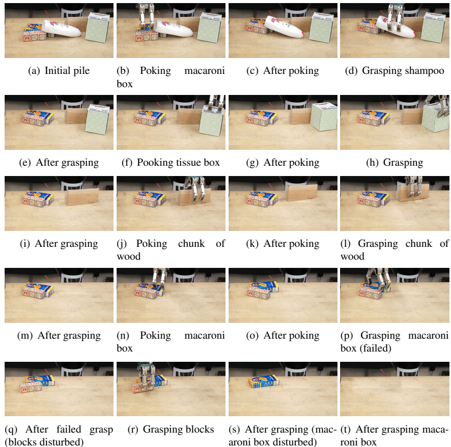
Figure 8: A sequence showing the performance of our algorithm with a pile of unknown objects: a tissue box, a chunk of wood, a bottle of shampoo, a box of macaroni, and toy blocks. The algorithm switches between pushing to verify segmentation hypotheses and grasping to remove objects from the table. Here, 10 actions are required to remove 5 objects. Videos are available at http://www.dubikatz.com/autonomousManipulation.html
