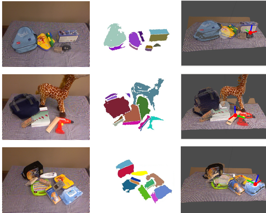
Figure 4: Experimental evaluation of facet detection. Left: pile on unknown objects. Middle: segmentation of the scene into facets (color coded). Right: 3D view of the scene. To interact with objects we instantiate compliant controllers with information extracted from each facet: COG (red circle) and principal axes (red = principal axis, green = secondary axis, blue = trinary axis).
